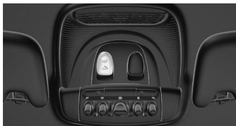
SOS button in the roofliner
